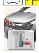
2. Raise the hood slightly, push the secondary latch up ② inside of the hood center and lift the hood (3)
